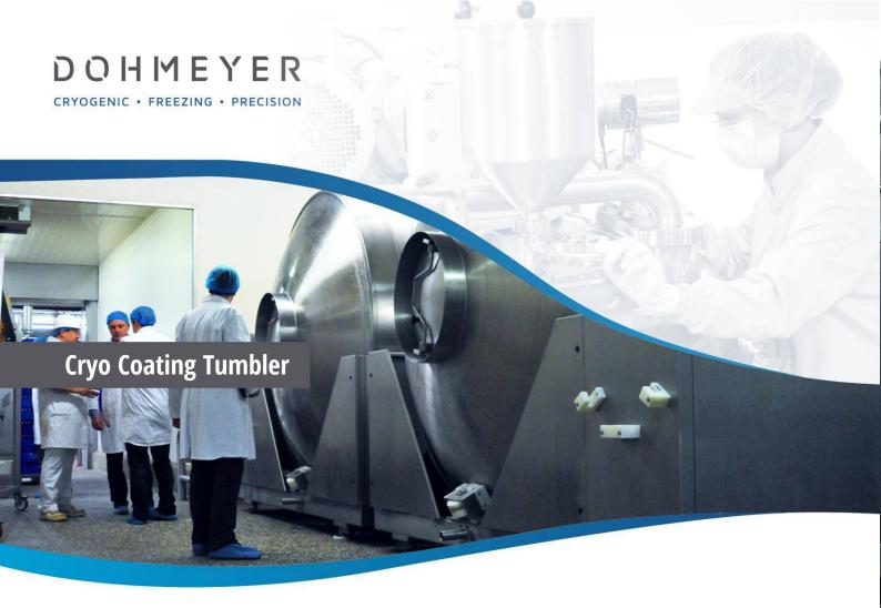
The **Dohmeyer Coating Tumbler**<sup>TM</sup> is the ideal solution for freezing small products by the individual quick freezing (IQF) processes in a batch production system. Like thinly sliced, diced or cut food products such as diced ham, sliced salami, diced/sliced chicken products, pizza toppings, shredded cheese, shrimps, diced cheese, sliced/diced vegetables, cut fruits and whole berries.
