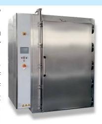
plunging into a nitrogen immersion bath. Cryogenic quenching offers a wide variety of advantages to your heavy duty components, as temperature is monitored, additional metallurgical transformations take place to relieve residual stresses, normalize and stabilize the metal alloy, increase resistance to wear, and create a modified and uniform crystal grain structure. The benefits of this process are increased part life, less wear, and improved performance.
