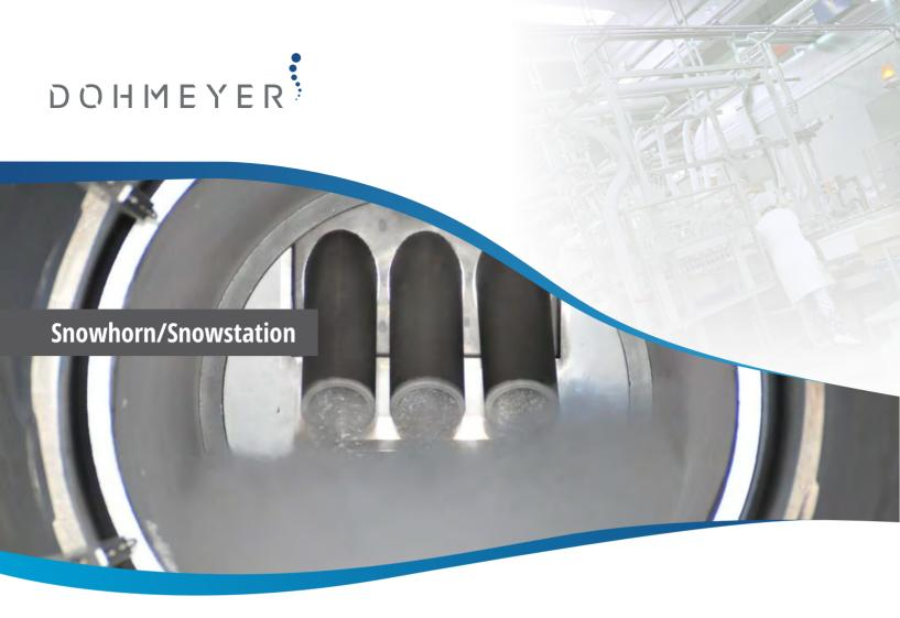
The Dohmeyer Snowhorn is developed as a versatile cooling device for a wide range of applications. Ranging from use in the cheese industry, the chocolate industry, the meat industry, among a wide variety of other sectors. The Dohmeyer Snowhorns are liquid CO2 only equipment systems, as if liquid CO2 tend to split in a gas and a solid (snow) fraction when it comes in contact with ambient atmospheric conditions.
