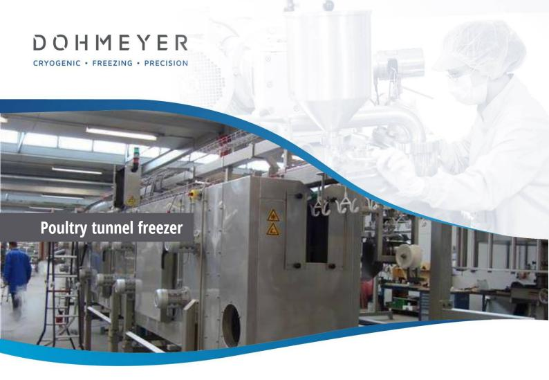
Dohmeyer combines research, development and in depth expertise to offer you the most efficient poultry freezer in the market. Our poultry freezer is capable of cooling down 4000 broilers an hour, allowing the outer skin to be averagely cooled down to -12°C on a depth of 3 mm. Scientific tests have also shown that liquid nitrogen reduces the CFU count of Campylobacter on the surface of the broilers offering a reduced microbiological activity on the exposed parts.
