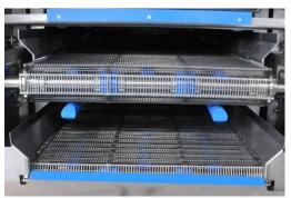
Every Dohmeyer **Multi-Deck freezer** is equipped with either liquid nitrogen or liquid carbon dioxide (CO2) injection, depending on the product and process requirements. The freezing action happens right inside the tunnel as the cryogenic gases are injected into an insulated cold zone as the product passes through it.
