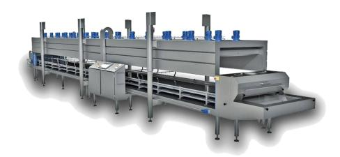
clearing and maintenance operations inside the tunnel. Every Dohmeyer Tunnel Dohmeyer Tunnel is equipped with either liquid nitrogen or liquid carbon dioxide (CO2) injection, depending upon the product and process requirements. The freezing actionhappens right inside the tunnel where thecryogenic gases are injected into an insulated cold zone as the food product passes through it.
