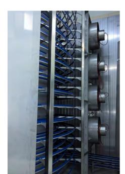
The Dohmeyer OptiFreeze<sup>™</sup> Spiralfreezer has a unique horizontal airflow design that maintains the same air temperature and air speed throughout all levels, minimizing residence time for the food products and reducing weight loss to obtain a higher yield. The horizontal airflow design generates flows up to 6m/s. The result is that every product, no matter of its location, is subject to the exact same airflow and therefore exits the freezer with a uniform temperature.
