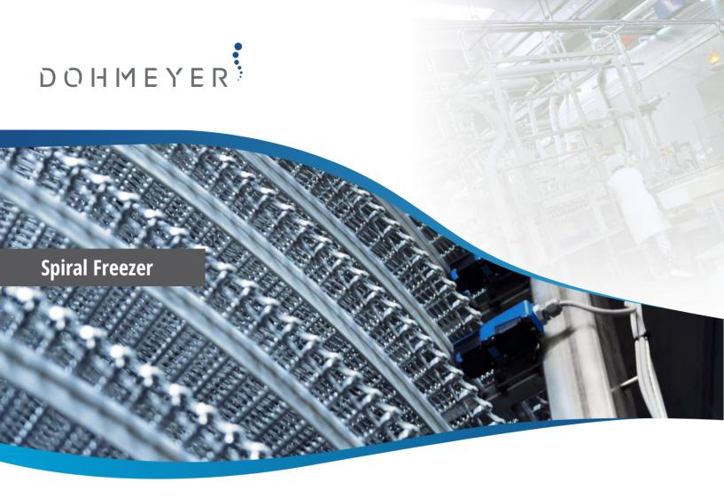
Dohmeyer's in-line Spiral freezers are commonly used to cool down or freeze large volumes of different food products ranging from pies, breads or even packaged, ready prepared meals.
