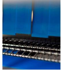
Liquid Nitrogen and CO2 deliver the ultimate in cryogenic freezingpower by minimizing any aroma flavour and dehydration losses to the food product. Because these cryogenic gases are inert, they also provide a protective atmosphere inside the freezing zone which prevents any oxidation of the food. As a result, the quality attributes of cryogenically-frozen food products are far more superior to those same products frozen in a mechanical system.
