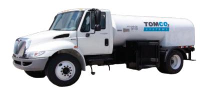
truck body for transporting high pressure cylinders in conjunction with a low-pressure bulk liquid CO2 delivery system weighs less than our standard DOT bodies. It also significantly reduces costs. The body's streamlined design is manufactured in accordance with DOT Title 49, Specification MC-331 and is available for 2.5 ton, 3 ton and 3.5 ton storage units.
