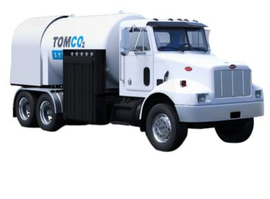
TOMCO2 System's economical truck body for transporting high pressure cylinders in conjunction with a low-pressure bulk liquid CO2 delivery system weighs less than our standard DOT bodies. It also significantly reduces costs. The body's streamlined design is manufactured in accordance with DOT Title 49, Specification MC-331 and is available for 2.5 ton, 3 ton and 3.5 ton storage units.
